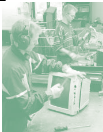
The MIREC recovery company separates tubes, plastic casings, glass and other components when dismantling TV/computer monitors. Photo: Peter Knutsson/El-Kretsen.
