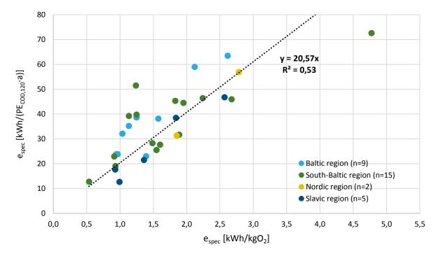
Figure 25 – Specific energy consumption kWh/kgO2 in relation to kWh/(PEcod, 120 a)
