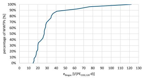
Figure 26 – Specific biogas production [l/(PEcod, 120 · d)], n=27
