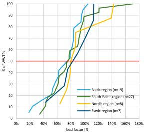
Figure 9 – Degree of utilization based on COD, regionalized
