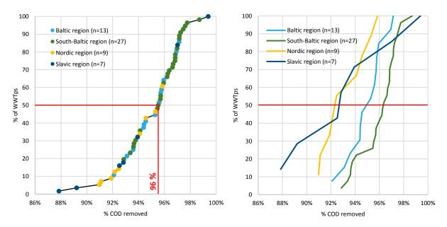
Figure 12 - Overall COD removal efficiency
