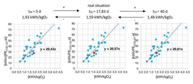
Figure 24 – Impact of sludge age on kWh/kgO<sub>2</sub>
