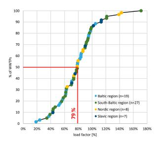
Figure 8 – Degree of utilization based on COD, accumulative
