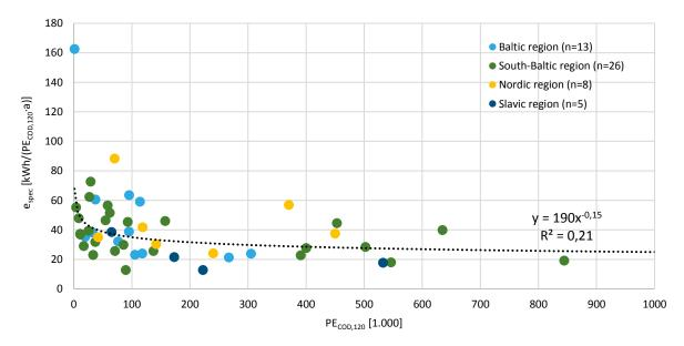
Figure 20 – Specific energy consumption [kWh/(PEcod, 120 · a)] in relation to connected PE [PEcod, 120 · a)]
