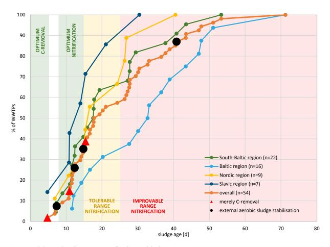
Figure 10 – Sludge age based on BOD₅ as overall and regional display
