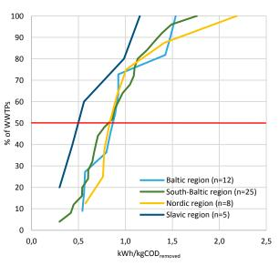
Figure 22 – Specific energy consumption [kWh/kgCODrem], accumulative
