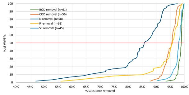
Figure 11 – Nutrient removal efficiency
