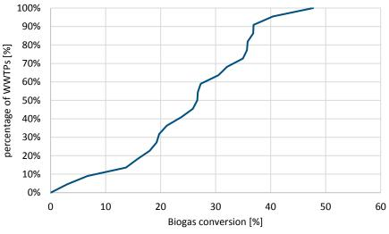
Figure 29 - Rate of biogas conversion into electrical energy, n=23
