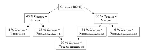
Figure 31 – Fractionation of the chemical oxygen demand according to Sieker [2018]
