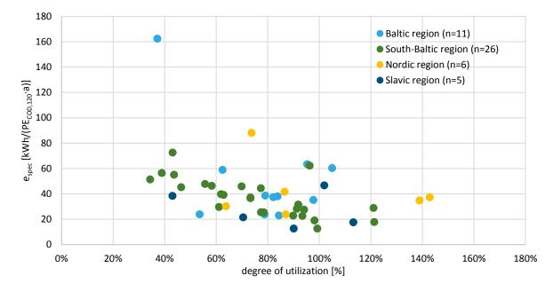
Figure 21 – Specific energy consumption [kWh/(PEcod,120·a)] in relation to degree of utilization
