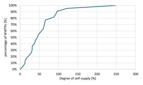
Figure 30 – Degree of self-supply of electrical energy, n=23
