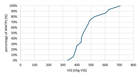
Figure 27 – Specific biogas production in relation to fed VSS [l/kg VSS], n=16
