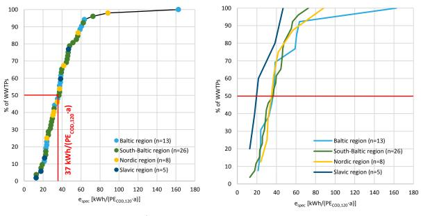
Figure 18 – Specific energy consumption [kWh/(PE<sub>cod,120</sub>·a)], accumulative
