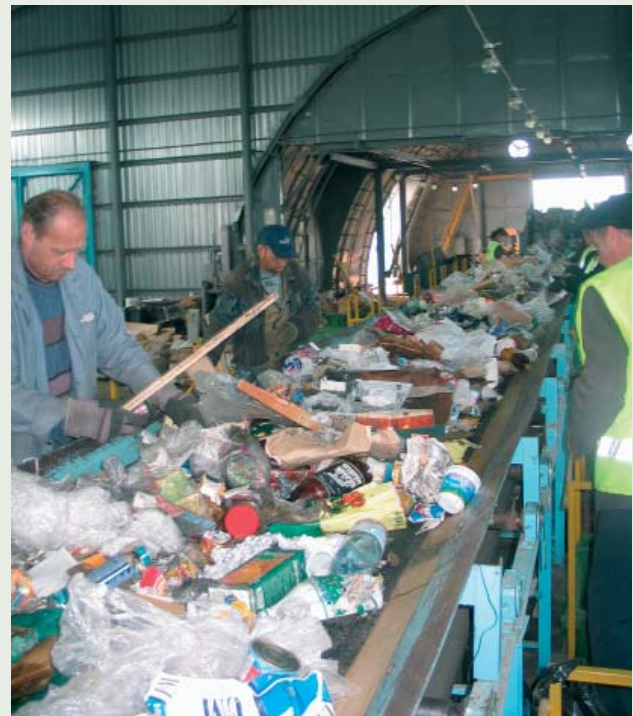
In St. Petersburg, a pipe line for sorting solid household wastes has been installed in one of the rubbish stations, which makes it possible to substantially reduce the volume of withdrawals, which are then directed to recycling.
